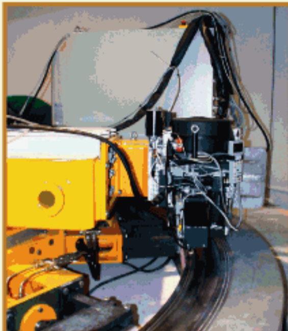
Zväracia hlava na makete jadrového reaktora Welding head located on the model of the nuclear reactor
